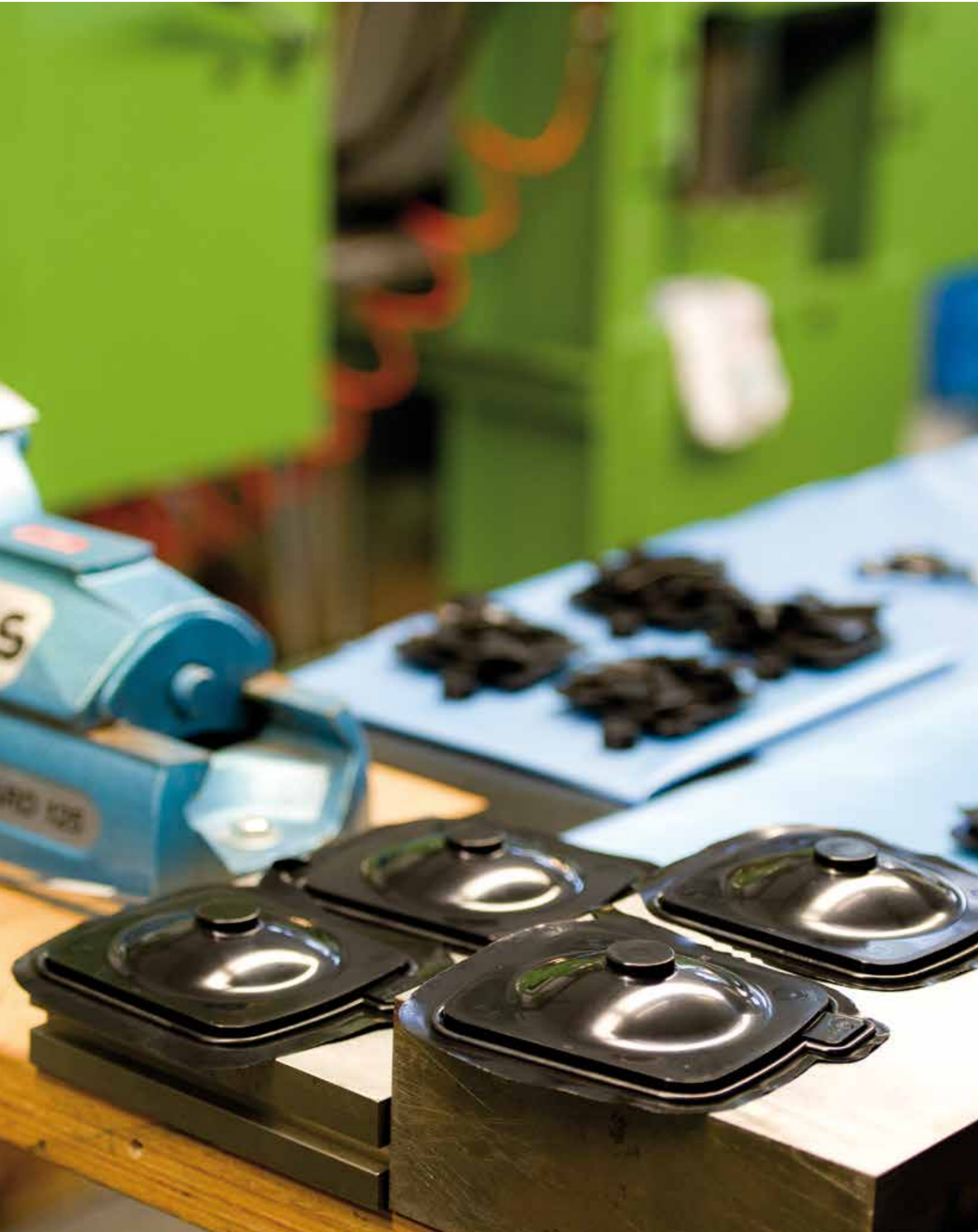
Diaphragm after vulcanisation, prior to trimming.
