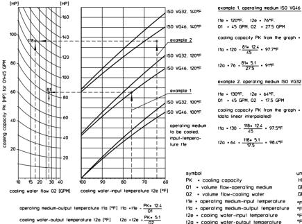
11e = 120°E 12e = 76°E 01 = 45 GPM, 02 = 27.5 GPM cooling capacity PK from the graph = 81 HP
