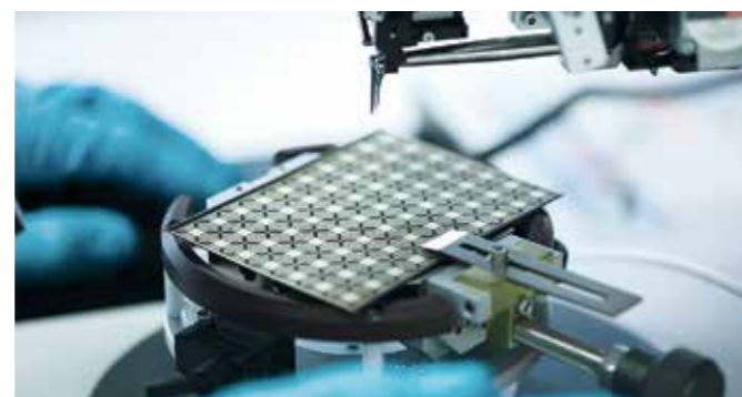
The test piece for the electrical connections is located under the manual bonder for the deep access wedge.
