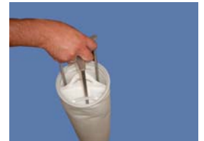
Photo 3: Insert the HAYFLOW installation tool in the element.
