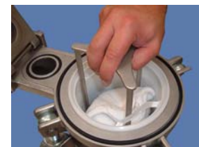
Photo 4: Push the element with the installation tool down to the bottom of the basket.
