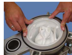
Photo 5: Push the HAYFLOW collar down.
