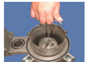
Photo 2: The lifting tool: Lifting up the basket.
