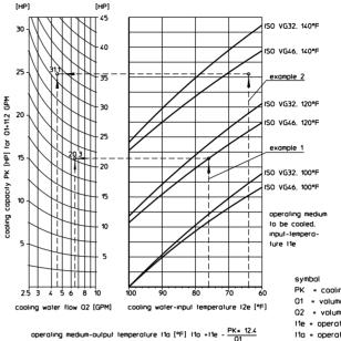
cooling water-output temperature 12a [°F] 12a = 12e +  $\frac{PK*5.1}{22}$
