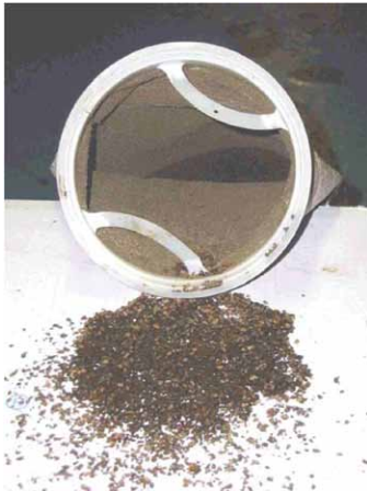
One #2 DURAGAF filter bag with collection of iron oxide "chip scale"
