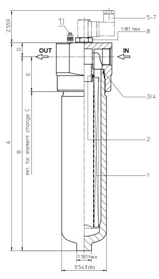
1) Connection for the potential equalization, only for application in the explosive area.
