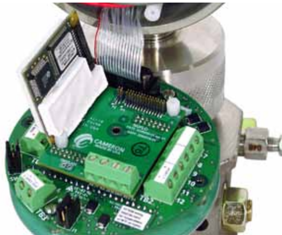
Figure 6.4—Removal of white potted fieldbus module
