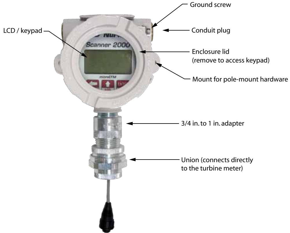
Figure 1.2—Scanner 2000 microEFM with turbine meter adapter
