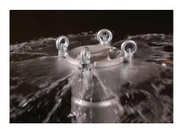
A broken or misplaced seal, a spike in line pressure, or the failure to fully relieve system pressure before servicing the vessel can result in a potentially dangerous and costly spray.
