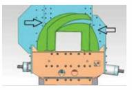
Clamshell #2 closes and compresses material for shearing/baling/ logging
