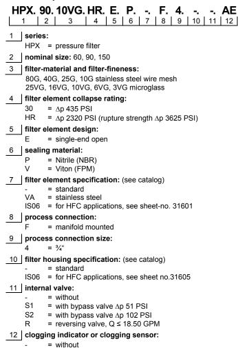
To add an indicator to your filter, use the corresponding indicator data sheet to find the indicator details and add them to the filter assembly model code
