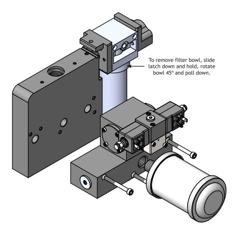
Valve packs may be quickly exchanged in the field. Locator pins provide positive valve alignment between the cylinder head and valve base.
