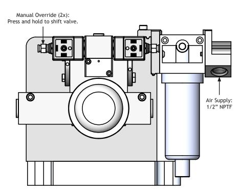
Air-filter (40 micron) promotes long life by removing pipe scale and other debris from the air-supply (1/2 NPSF).
