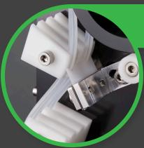
Acetyl scraper with adjustable horizontal movement allows you to set a light scraping pressure.
