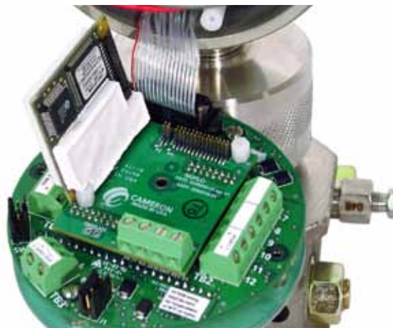
Figure C.10—Removal of white potted fieldbus module
