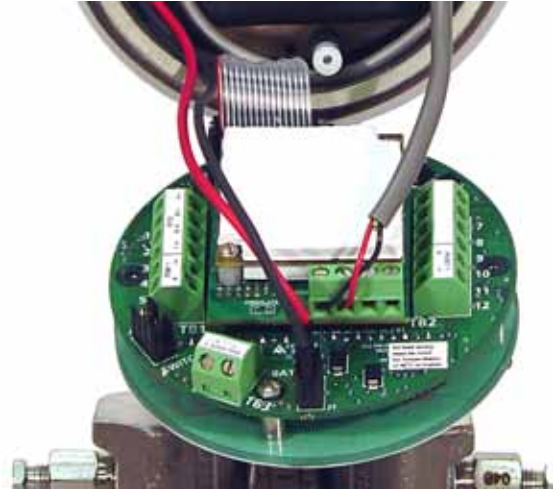
Figure C.9—Removal of the battery cable and fieldbus interface board cable
