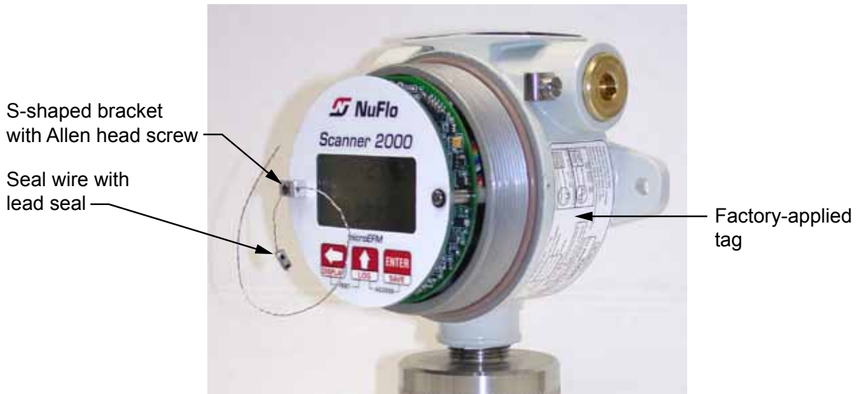
Figure A.20—Measurement Canada seal kit components
