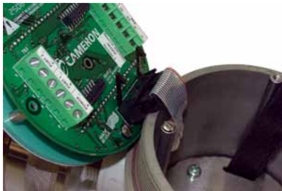
Figure 5.2—Latch securing the ribbon cable
