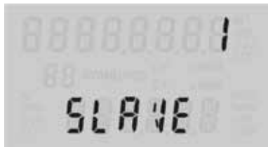
Figure 1.9—In configuration mode, the parameter to be configured is displayed at the bottom of the LCD and the setting for that parameter is displayed in the top LCD.
