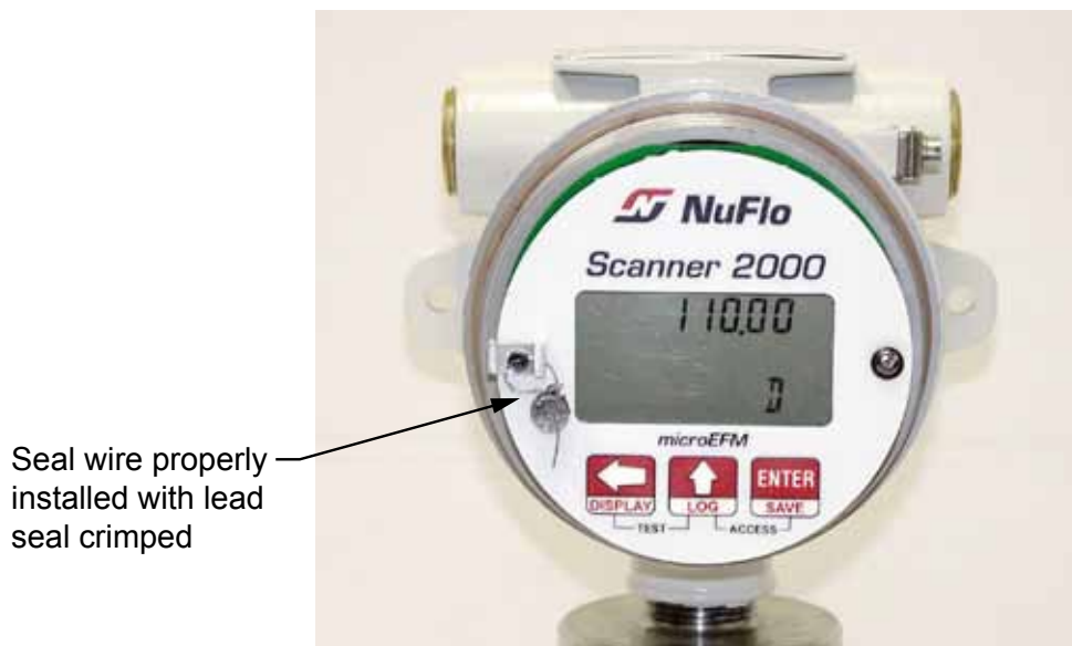
Figure A.21—Scanner 2000 with seal kit installed
