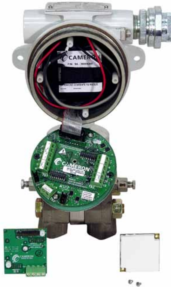
Figure C.11—Removal of the fieldbus interface board
