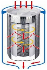
Internal view of filter element
